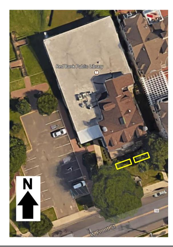
**BIORETENTION SYSTEM:** Rain gardens can be used to reduce sediment and nutrient loading to the Navesink River and increase groundwater recharge. Two rain gardens can be installed in front of the library to capture, treat, and infiltrate runoff from the downspouts in front of the building.
